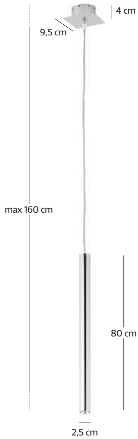
art. Stiled S 80 LED 3 W Lente 60° 3000 K 160 lm - Driver incluso / Driver included
